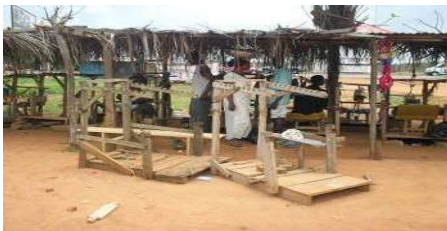
Structure of a single heddle craft loom.
